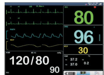
Max 8 waveform display simultaneously max 6 leads ECG waveforms display
