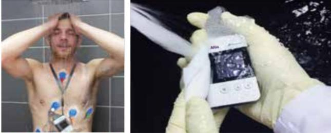
The Holter Recorder reaches protection grade up to IP27, intending to prevent unexpected damages from water or dust, which maximizes patients' freedom in their daily life, even in their shower time. At the same time, it facilitates the cleaning and sterilization procedure.
